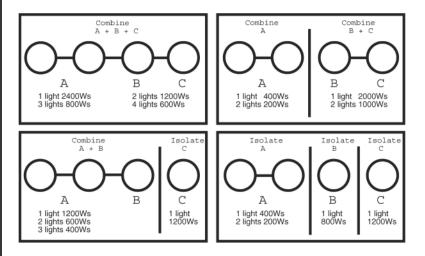
Divide watt-seconds by 2 when using half power (-1 stop). Divide watt-seconds by 4 when using quarter power (-2 stop).
